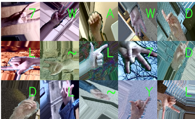
Fig. 8. Image processing operations applied to the training images include color-shift, zoom, shear, rotation, axes flip and position shift processes.
