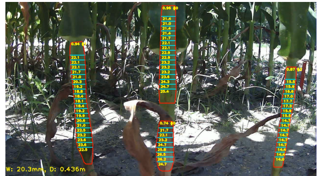
Figure 3: A visualization of the corn stem width algorithm on a 2021 corn field. Masks are annotated with estimated width in millimeters at several points.
