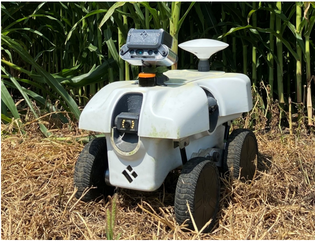
Figure 1: EarthSense TerraSentia robot is a compact robot designed to collect under-canopy traits in an autonomous manner. We built over 100 such robots in 2021. In this paper we describe results for high-throughput phenotype estimation in corn and soybean using data from these robots.
