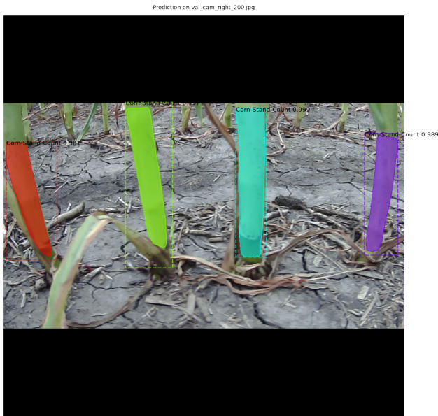
Figure 4: A visualization of the corn stand count detector fed into the stand count algorithm. Masks are annotated with confidence.
