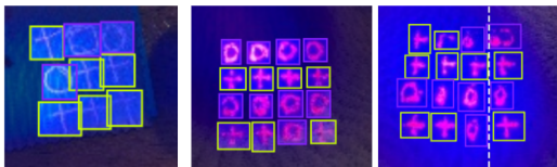
Figure 5 – fabrics marked with circles and crosses, visible under blue light, and marked with bounding boxes for reading by an object detection algorithm.
