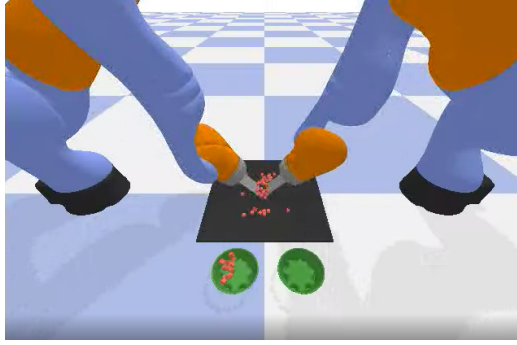
Figure 11: An example of the camera image for the bi-manual sweep robotic-arm manipulation task.
