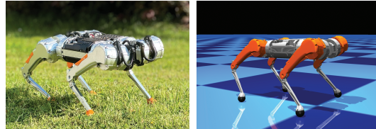
Figure 2: MAB Robotics HoneyBadger quadruped robot in the real world (left) and in the MuJoCo simulation (right).
