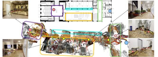
Fig. 6: Real-world Validation Result . Exploration process of a quadrupedal robot in a real-world environment. Top: Floor plan. Bottom: Reconstructed map and exploration path from TSDF integration using monocular depth prediction. Colored boxes indicate key correspondences between the map and floor plan.
