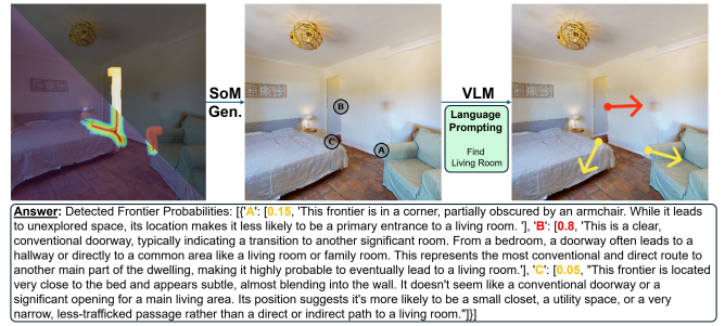
Fig. 3: VLM-based Extension of FrontierNet. OpenFrontier takes the 2D frontier clusters produced by FrontierNet and queries a VLM using set-of-mark prompting. This re-weights the information gain of each frontier based on a given language instruction, grounding vision-language understanding into detected frontiers. In practice, we merge these relevance weights with the information gain predicted by FrontierNet, allowing the system to balance task-driven exploitation with exploration.
