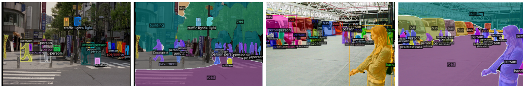
Figure 3: Qualitative results for object detection, segmentation and panoptic segmentation on COCO val as generated by SimPLR with ViT-B backbone. SimPLR can detect and segment objects in crowded scenes.
