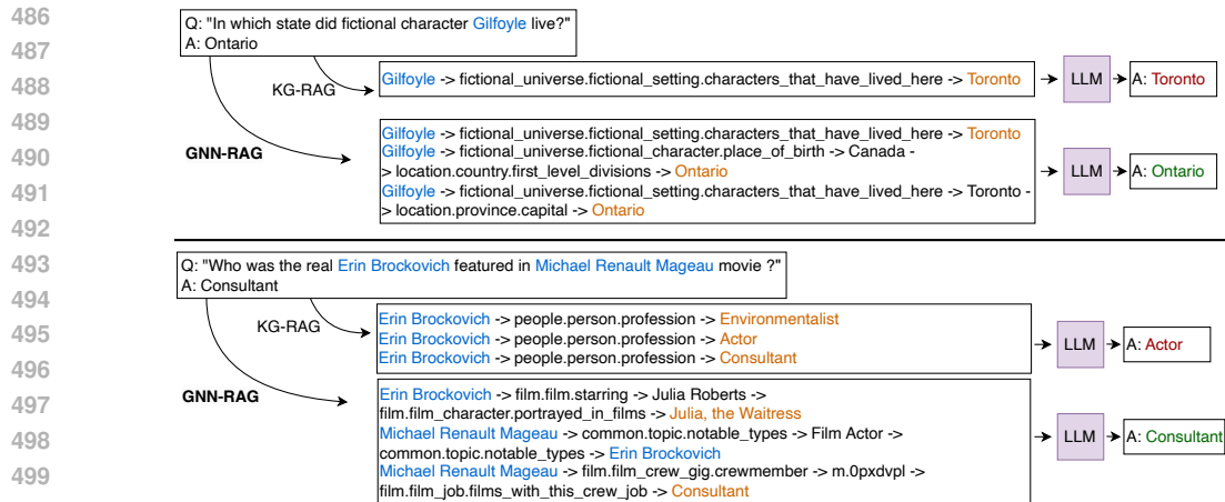
Figure 5: Two case studies that illustrate how GNN-RAG improves the LLM’s faithfulness. In both cases, GNN-RAG retrieves multi-hop information that is necessary for answering the complex questions.
