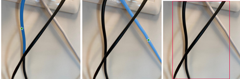
(a) An example of unsuccessful segmentation with a single point. (b) An example of successful segmentation with a single point. (c) An example of box prompt for DLO segmentation.
