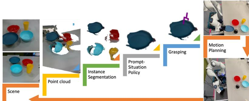
Figure 8: Pipeline for Real Hardware Experiments
