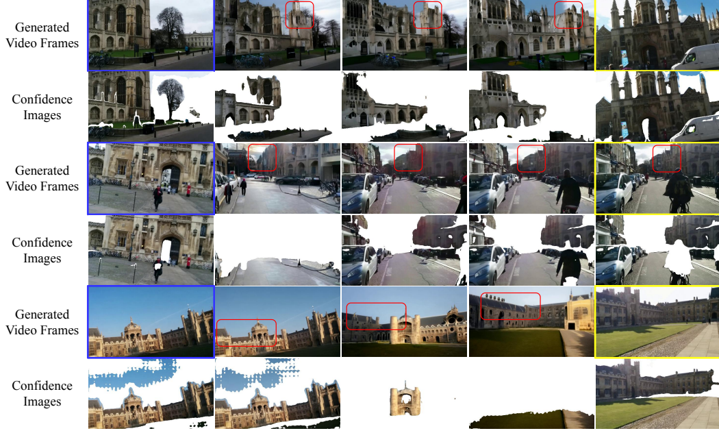
Figure 4: Hybrid Video Generation artifacts under severe illumination differences. Blue and yellow outlines indicate the start and end frames, respectively. Confidence images denote images filtered with the predicted confidence map in the subsequent DUS3R model. The red boxes highlight regions affected by artifacts in these cases. We can observe that these regions have quite low confidence.
