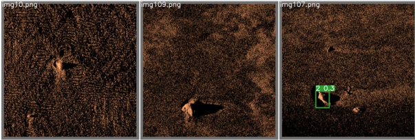
Figure 5. YOLOv7_tiny model trained with FLS images, tested on SAS images from the SASOptical dataset
