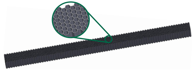
Figure 3: 3D CAD model of laminar airflow former, passage for high-pressure air from the fans to make the fog exit in a particular direction to form a flat screen. Taking a closer look at the airflow former design, it is similar to gluing a series of plastic straws together by the side or like a honeycomb.
