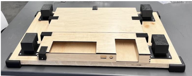
Fig. 2. Additional shell showcasing the underside of the board before introduction of electrical components & LattePanda.
