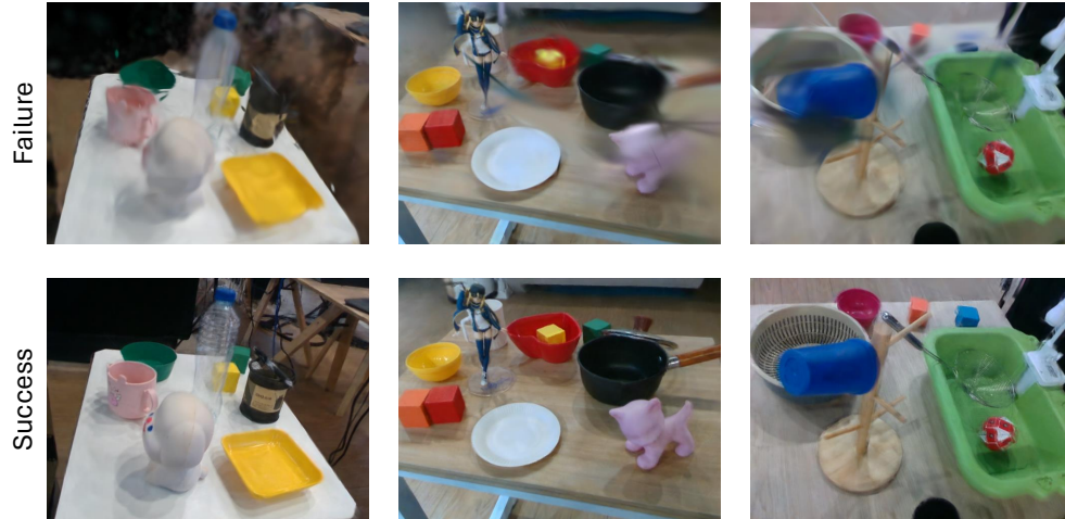
Figure D1: The comparison of reconstruction failure caused by camera jittering and the successful results.
