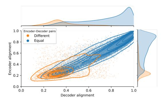
Figure 1: Cosine similarities of latents from SAE 1 with their counterparts in SAE 2. Both SAEs have 32K latents, and are trained on the sixth MLP of Pythia 160M. Contour lines are regions of equal density according to kernel density estimation. We color each SAE 1 latent depending on whether the encoder-based and decoder-based matchings agree on which counterpart it should get.
