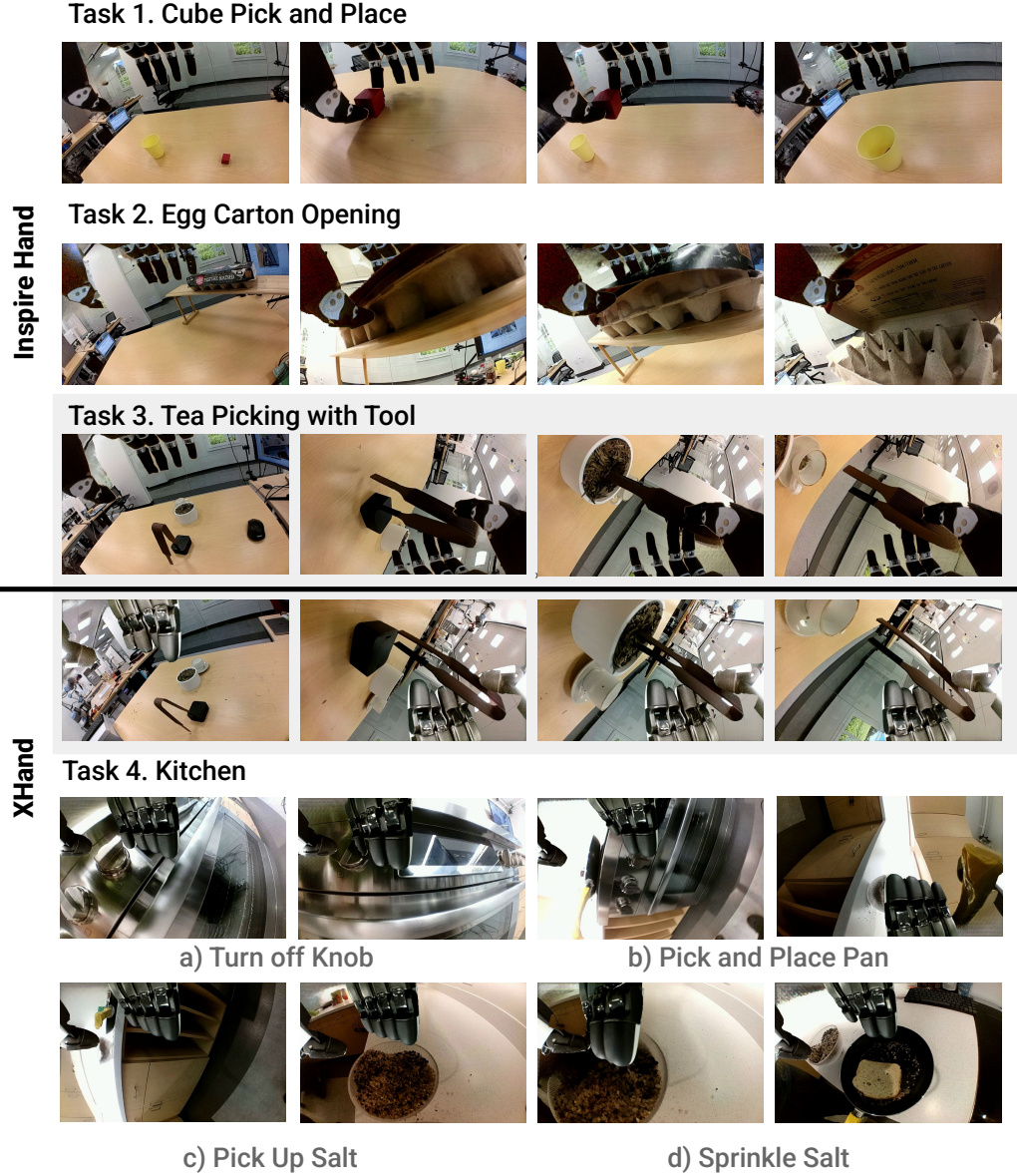
Figure 7: Inpainting Results. The visual observations in the original collected dataset contain exoskeletons and human hands. The software adaptation layer replaces these pixels with corresponding robot hand images while preserving the natural occlusion relationships during hand-object interactions. Please see project website https://dex-umi.github.io for details.
