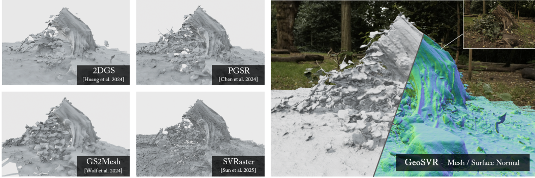
Figure 1: Geometric Sparse-Voxel Reconstruction. Our method, abbreviated as GeoSVR, delivers high-quality surface reconstruction for intricate real-world scenes based on explicit sparse voxels. Our superiority is exhibited compared to the state-of-the-art approaches built upon Gaussian Splatting, which encounter rough, inaccurate, or incomplete recovery problems even with help from external estimators, excelling in delicate details capturing with high completeness and top-tier efficiency.
