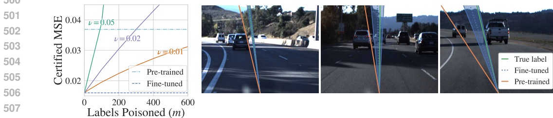
Figure 5: Left: Fine-tuning PilotNet on unseen data with a bounded label poisoning attack ( q = \infty ). Right: Steering angle prediction bounds after fine-tuning ( m = 300, q = \infty, \nu = 0.01 ).
