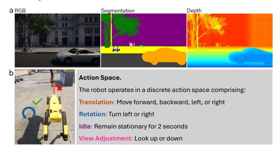
Figure 8: **Multimodal observation and discrete action space**.(a) The robot perceives the environment via RGB, segmentation, and depth modalities. (b) Its action space includes translation, rotation, idling, and view adjustment.
