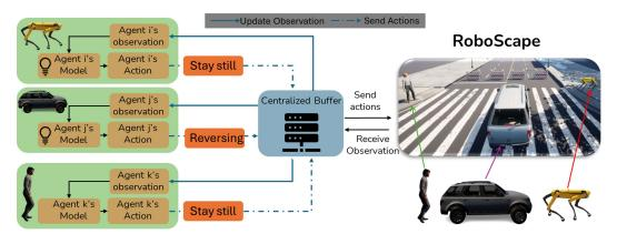
Figure 7: **Asynchronous multi-agent control.** To ensure each agent independently selects and executes actions based on its local observation and policy model, a centralized buffer serves as the interface between agents and the environment, receiving actions from all agents and updating their observations based on the resulting environmental changes.
