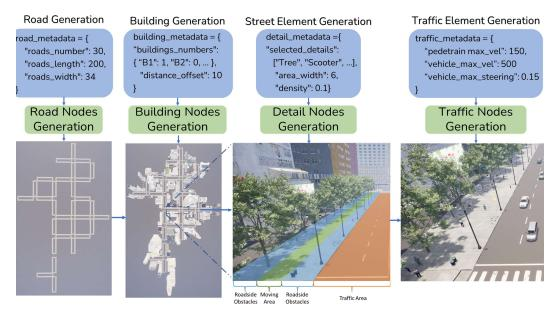
Figure 3: **Procedural City Generation.** SWR receives a user's specification and modularizes the process into road, building, details, and traffic elements generation.
