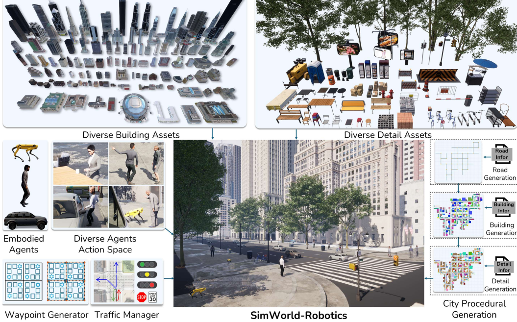
Figure 1: Overview of SimWorld Robotics (SWR). Built upon Unreal Engine 5, SWR is a simulation platform for large-scale, photorealistic, and dynamic urban environments. It offers diverse high-fidelity building and object assets, supports embodied agents with rich action spaces, includes a background traffic system powered by city-scale waypoint generation, and enables comprehensive city procedural generation.
