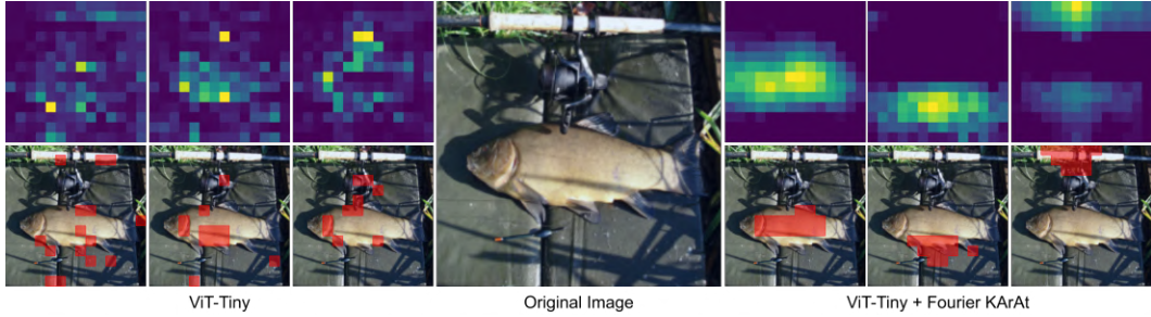
Figure 11: ViT-Tiny attention map characterization. Original image for inference (the center), the attention maps (top row), and contributing image regions (bottom row) for all three heads in ViT-Tiny: traditional MHSA (left) and Fourier KARAt G_3B (right). The traditional MHSA sporadically focuses on fine-grained features of the primary object in the image. In contrast, the learnable attention in Fourier KARAt identifies the primary object features present significantly across all heads.
