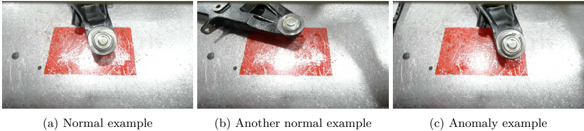
Figure 2: Examples of normal and anomaly images of a circular pin assembly obtained from Anonymous Corporation.
