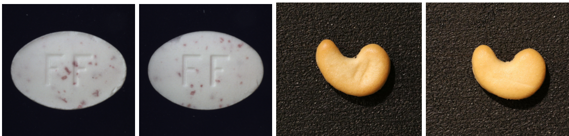
(a) Normal example of a pill, but there is a noticeable chip on the right of the pill. (b) Anomaly example of a pill, with a similar sized chip on the top of the pill. (c) Normal example of a cashew, with a scratch that seems less prominent than the normal image in (c). (d) Anomaly example of a cashew, with a scratch that seems less prominent than the normal image in (c).
