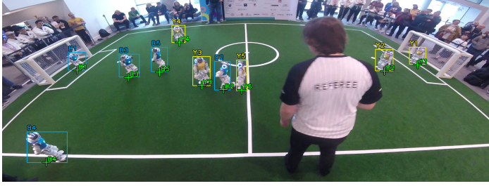
Figure 2: Visualization of robots identified by the tracker. The tracking result is represented by bounding boxes and IDs at their top. Ground truth positions are represented by green crosses and corresponding green IDs.
