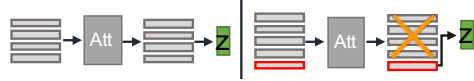
Figure 3: Multi-head attention-based encoder. Left. Regular sequence-to-sequence translation, each element of the output sequence is used. Right. An additional compression token is added to the sequence. From the output sequence, only the compression token is taken.
