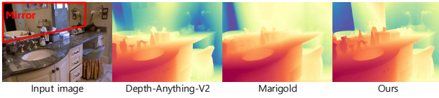
Figure 9. Failure cases in depth estimation. Red and Blue areas indicate near and far depth predictions, respectively.
