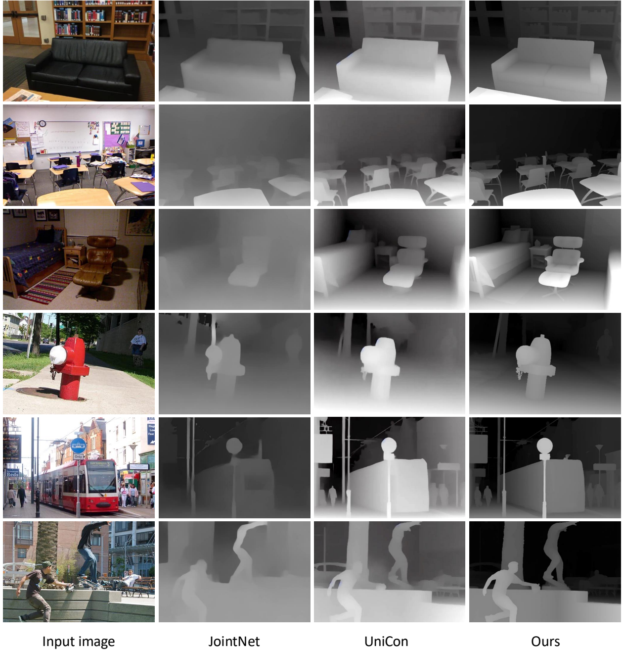
Figure 13. Depth estimation results of joint generation models. We visualize the depth estimation results of JointNet, UniCon, and our method on the NYUv2, ScanNet, MSCOCO dataset [17, 38, 56]. Our method shows sharp and fine-detailed depth visualization, which aligns with the trends observed in the qualitative results.
