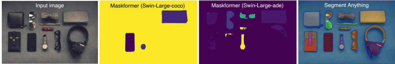
Figure 16. Challenge segmentation examples. To streamline segmentation tasks, we utilize the MaskFormer model (Cheng et al., 2021) trained on the COCO (Lin et al., 2014) and ADE20K (Zhou et al., 2017) datasets, along with the Segment Anything (SAM) model (Ma & Wang, 2023). We observe that MaskFormer occasionally under-segments, whereas SAM is prone to over-segmentation. Consequently, manual adjustments are necessary to ensure the datasets are accurately prepared for evaluation.
