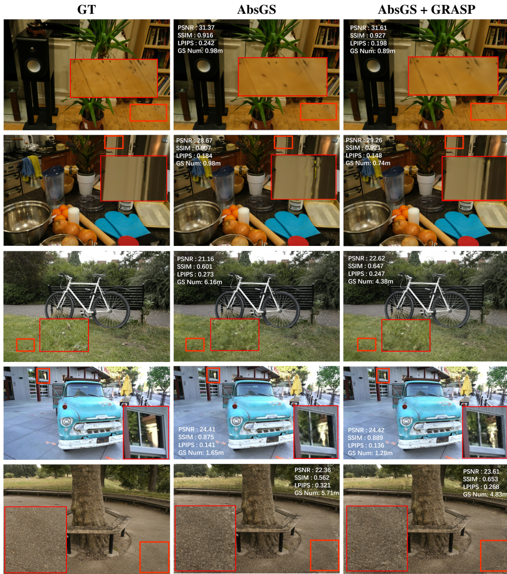
942 943 944 945 946 947 948 949 950 951 952 953 954 955 956 957 958 959 960 961 962 963 964 965 966 967 968 969 Figure 8: GRASP integrated with AbsGS. The geometric initialization and saliency pruning mod- 970 ules of GRASP can be effectively integrated into other Gaussian Splatting frameworks. Quantitative 971 improvements are shown in Table 1, with consistent gains in PSNR, SSIM, and LPIPS while reduc- ing Gaussian counts.
