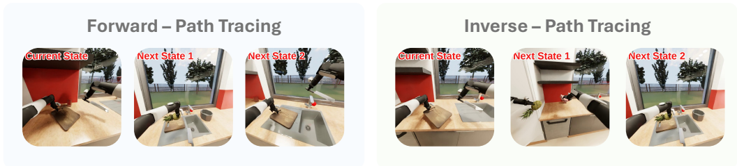
Figure 20: The figure illustrates Forward World Modeling (left) and Inverse World Modeling (right) trajectories rendered using the path tracing engine in NVIDIA Isaac Sim.
