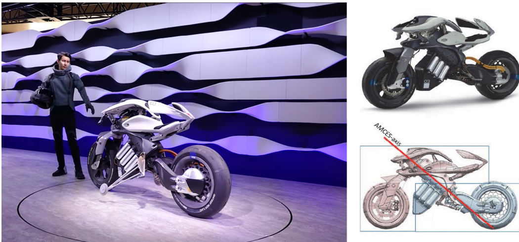
Figure 5: Yamaha's "MOTOROiD" is a shape changing, self-balancing motorcycle [52]. Its unique twisting chassis is able to affect the ride feel in real time as well as drive autonomously.
