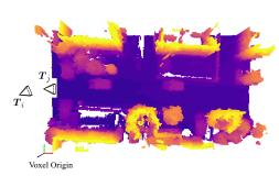
Figure 6: An illustration of the coordinate system transformation is provided in the bird's-eye view of the occupancy ground truth. Specifically, it depicts the transformation from the voxel coordinate system associated with the j-th frame to the camera coordinate system of the i-th frame. This transformation enables subsequent computation of the frustum mask and the visibility mask.
