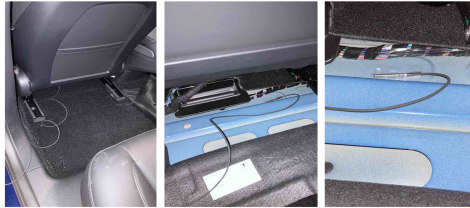
Figure 3: Installation of the sensor on the floor of the cabin.
