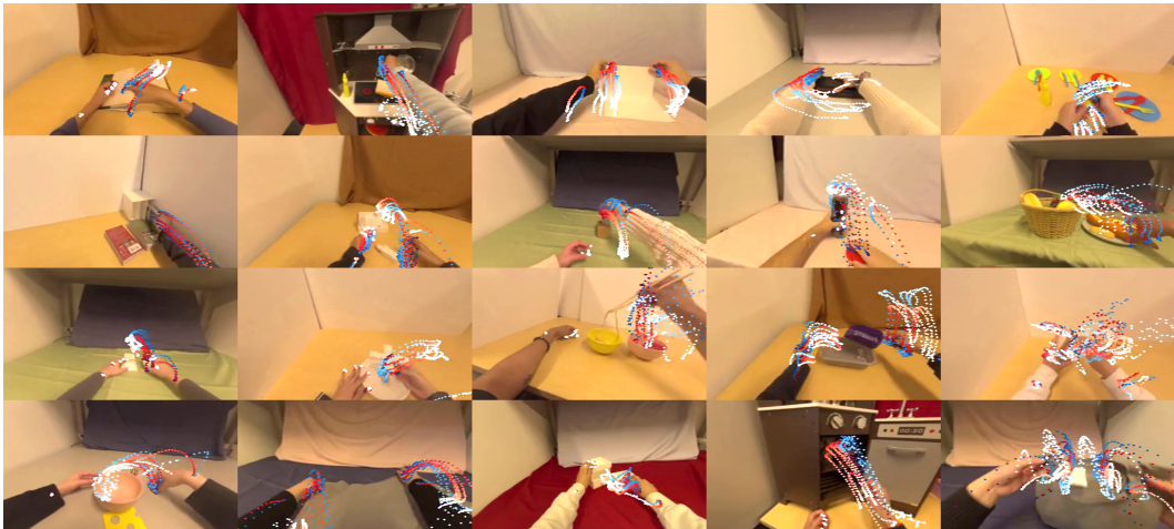
Figure 4: Model prediction visualizations for Dec + BC on test set images with a 2 second horizon. Blue trajectories are ground truth and red trajectories are predictions , where darker colors and closer to the current frame and lighter colors are further in the future. The points shown are the wrist and fingertip positions projected into the camera frame (a total of 12 trajectories).
