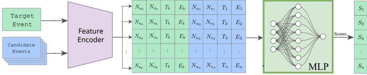
Figure 1: Visualization of the inner structure of the Parameterized Graph Explainer (Luo et al., 2020) adapted for the temporal graph setting. The input representation (source node features, target node features, event time features, and edge features) of the target event is concatenated with the representations for all candidate events considered.
