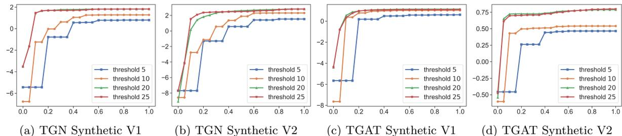
Figure 5: Fidelity-sparsity curves for the two target models on the synthetic datasets, at considered candidate events threshold (5, 10, 20, 25). The performance of the explainer grows proportionally with the number of candidate events until 20 but the performance at 25 candidate events is only marginally better than at 20.
