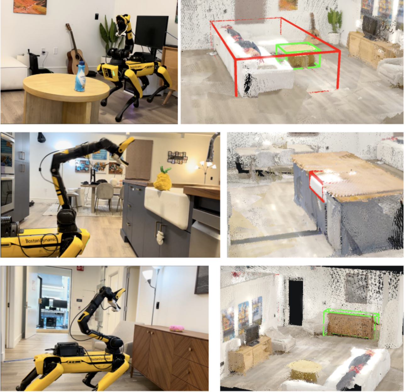
Figure 12: Examples of the Spot robot at the end of navigation task before the pick task (right) the output bounding boxes of LOCATE 3D+ model (left). The task (top) "navigate to coffee table in front of the sofa and pick up the bottle" (middle) "navigate to sink and pick up the pineapple plush toy" (bottom) "navigate to the dresser in the hallway and pick up pink plush toy"
