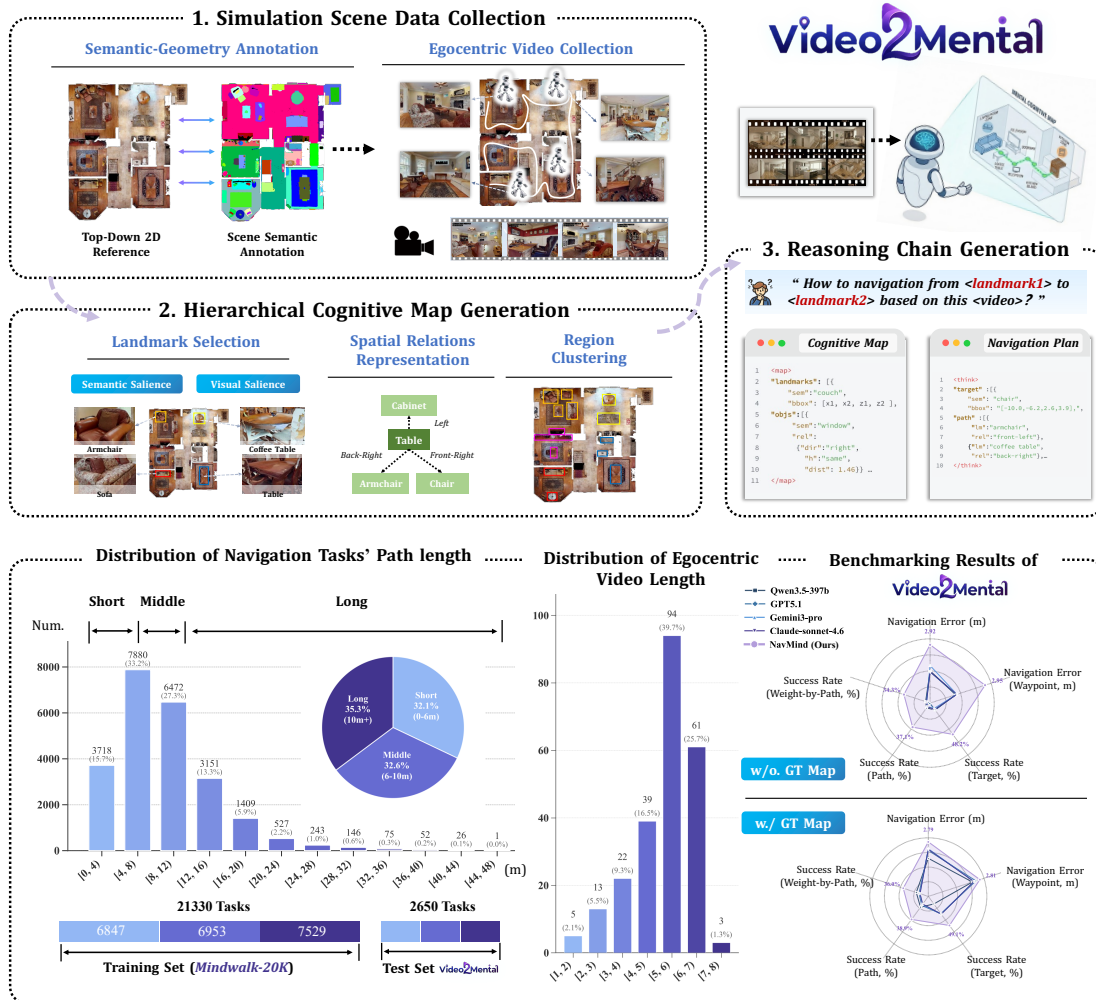
Figure 2. Data generation pipeline and benchmark analysis. Video2Mental Benchmark Construction and Statistics. We collect simulator-based semantic annotations and egocentric exploration videos, synthesize hierarchical cognitive maps via rule-based landmark selection, and extract landmark-grounded path planning sequences. The resulting dataset contains over 24k mental navigation tasks with average path lengths exceeding 9 meters and more than 80% of videos longer than 4 minutes. Preliminary evaluations show that existing MLLMs struggle to demonstrate genuine mental navigation capability.
