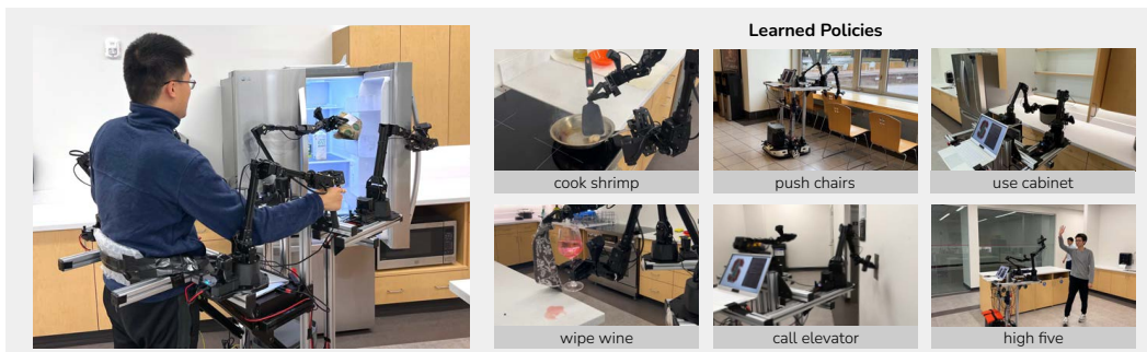
Figure 1: Mobile ALOHA . We introduce a low-cost mobile manipulation system that is bimanual and supports whole-body teleoperation. The system costs $32k including onboard power and compute. Left : A user teleoperates to obtain food from the fridge. Right : Mobile ALOHA can perform complex long-horizon tasks with imitation learning.
