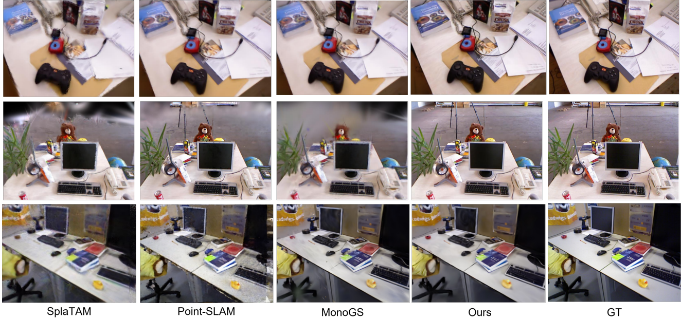
Figure 4. Rendering results on the TUM dataset. The proposed keyframe-triggered single-step initialization produces sharper edges, fewer transparency artifacts, and more consistent colors than residual-driven densification.
