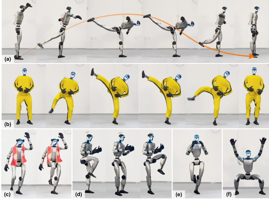
Figure 1: Extreme Balance Tasks. HuB enables humanoids to perform extreme quasi-static balance tasks with high stability. (a) Swallow Balance: holding a challenging T-shaped pose with the torso extended horizontally; (b) Bruce Lee’s Kick: executing a high kick with full leg extension while balancing on one foot; (c) Ne Zha Pose: a martial arts-inspired one-legged stance with a raised arm; (d) High Knees; (e) Single-Leg Stand; (f) Deep Squat. Videos are available at: hub-robot.github.io
