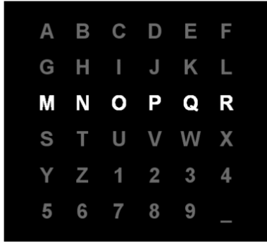
Fig. 1. The 6×6 P300 display paradigm used for recording the dataset. One of the rows is intensified in the presented image.
