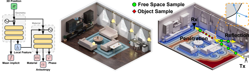
Figure 2: RF Ray Tracing with Neural Representation.
