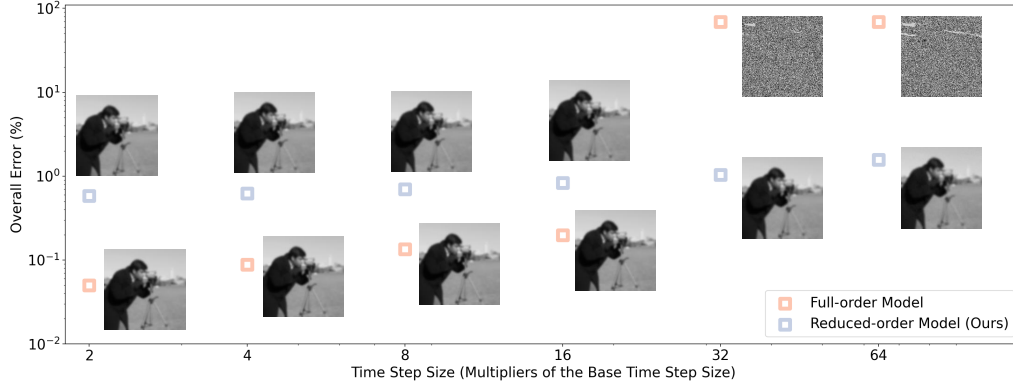
Figure 35: Stability analysis. We systematically increase the time step size ( \Delta t ). Our method remains stable in a wide range of time step size and maintains an error close to 1%. By contrast, the full-order model (that was used for training data generation) goes unstable as the time step increases and suffers from major visual artifacts.
