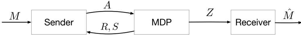
Figure 2: A depiction of the structure of MCGs. First, the sender is given a message. Second, the sender is tasked with a MDP, unrelated to the message. Third, the receiver observes the sender’s trajectory. Fourth, the receiver estimates the message.
