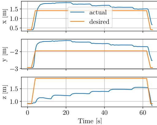
(a) REAL reducing position errors across the  $x$ ,  $y$ , and  $z$ -axes under unmodeled dynamics: In this experiment an additional weight of 210 g was added to one of the UAV's arms, creating a large unmodeled external torque that affects the attitude and position control of the UAV. REAL identifies the correct APIs to reduce this error, though convergence is slowed down due to the limited rate at which the API can be called.
