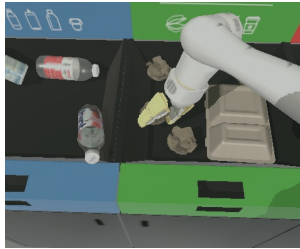
Figure 5: In the simulated vision-based robotic grasping tasks, a robot arm must grasp various objects placed in bins in front of it. Full implementation details are described in Appendix A.1.2.
