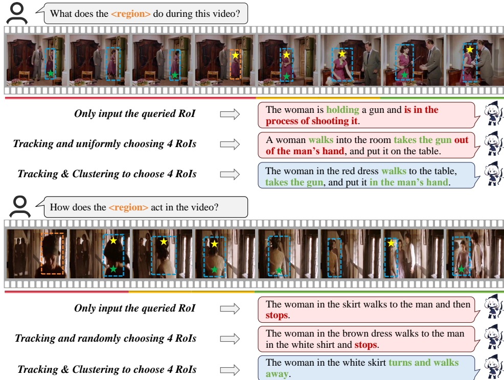
Figure 5: How RoI tracking and selection gradually improves the quality of video-based referring. In each example, the orange rectangle indicates the input <region>, blue rectangles are the tracked RoIs, and green and yellow stars label the uniformly sampled and K-means selected RoIs, respectively. Red and green texts highlight the incorrect and correct outputs. This figure is best viewed in color.
