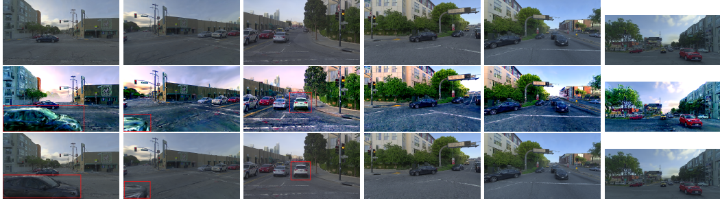
Figure 6: Asset insertion to achieve traffic densification. Multiple assets (black SUV and white car marked in red) are extracted from Pandaset scene “002” (source scene) and inserted into Pandaset scene “001” (target scene). (Top row) Multicamera renderings for a frame from the target scene. (Middle row) Asset insertion with source and target scenes trained using SplatAD. (Bottom row) Asset insertion with source and target scenes trained using AstroSplat. Unlike SplatAD, AstroSplat enables high fidelity asset transfer.
