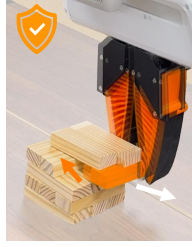
Fig. 5: Teleoperator Playing Jenga with Safety Filters. UNISafe enables non-conservative yet effective filtering of the teleoperator’s actions, ensuring the system remains within the in-distribution regions. In contrast, the uncertainty-unaware safety filter LatentSafe optimistically treats uncertain actions as safe, leading to failure.
