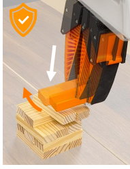
Fig. 5: Teleoperator Playing Jenga with Safety Filters. UNISafe enables non-conservative yet effective filtering of the teleoperator’s actions, ensuring the system remains within the in-distribution regions. In contrast, the uncertainty-unaware safety filter LatentSafe optimistically treats uncertain actions as safe, leading to failure.
