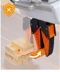
Fig. 5: Teleoperator Playing Jenga with Safety Filters. UNISafe enables non-conservative yet effective filtering of the teleoperator’s actions, ensuring the system remains within the in-distribution regions. In contrast, the uncertainty-unaware safety filter LatentSafe optimistically treats uncertain actions as safe, leading to failure.
