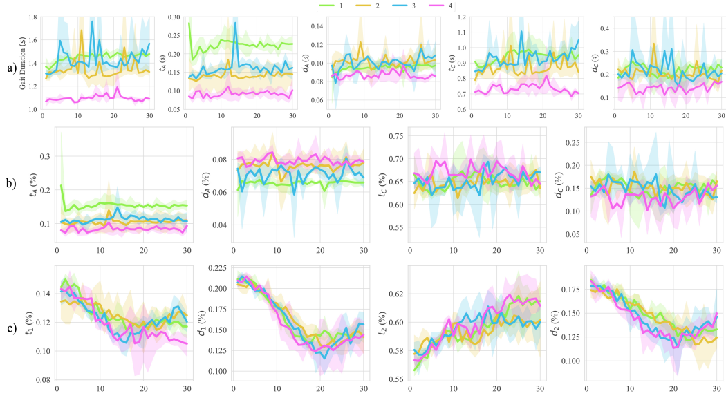
Figure 7: Characteristic timings and durations of gait trials: a) Raw gait data in seconds during training. b) Respective RIIV-processed data. c) RL policy during training. The shaded regions represent the 95 % confidence range of the three experiment trials. The x-axis is the number of gaits.
