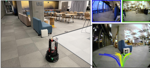
Figure 2: Visualizing the task-agnostic (yellow) and goal-directed pathways for two goal images (green, blue) learned by NoMaD.
