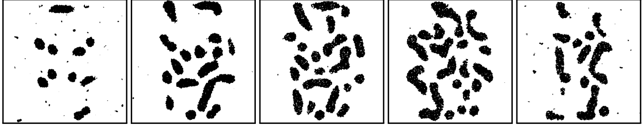
Figure 7. Cross-sectional slices of a genus 5 object with Voronoi mesh displacement mapping and 3 octaves of 3D Perlin noise.
